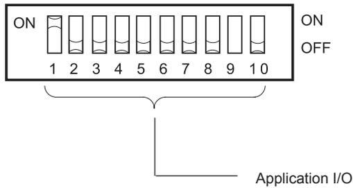
The DIL switches can be read from the STRATON application program and can be used for simple end user configuration.
